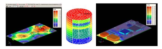
• ASONIKA-T performs modeling of stationary and non-stationary heat transfer in arbitrary combination of connected radio-electronic devices mechanically connected as modules in an integrated set of equipment.
