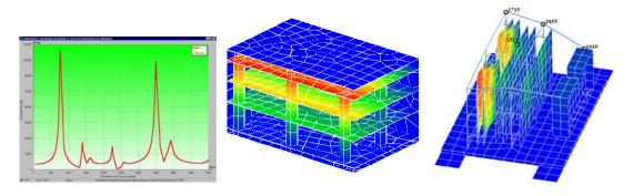
ASONIKA consists of series of modules, which can exchange data via a common interface. Each module can operate as independent computer program designated for solving the special tasks related to the device design and computing its properties. Each module has its own data base of materials, which can be expended and modified in a dialogue mode:
